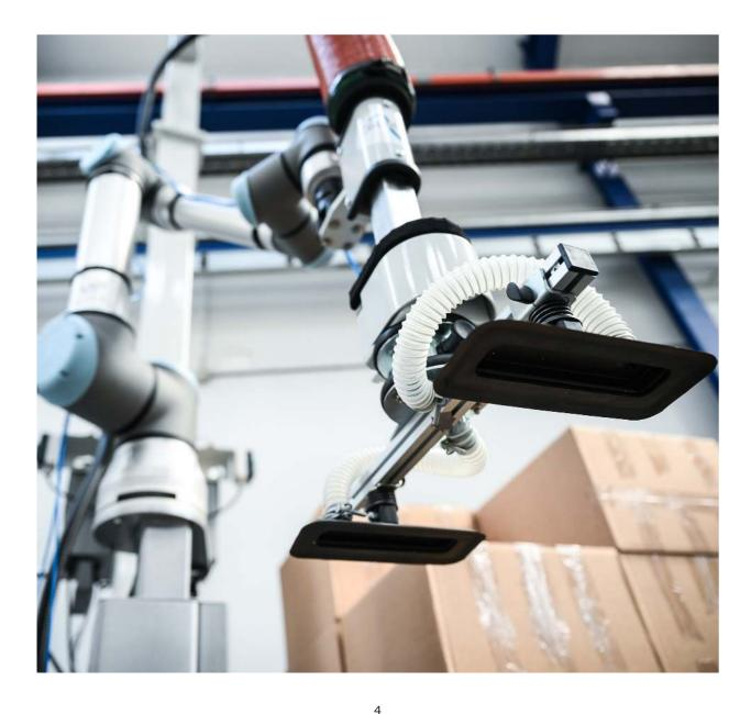
Integrates robot, controller, teach pen- with the robot. This solution permits condant, vacuum tube and pump and also tinuous operations and operator can easily crane in a single unit for maximum flexi- remove one complete pallet without stopping bility and mobility. a collaborative robot. Given solution can be moved with a lifter.
